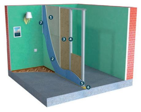
airborne noise 62 R "≈ insulation index of the entire structure dB
