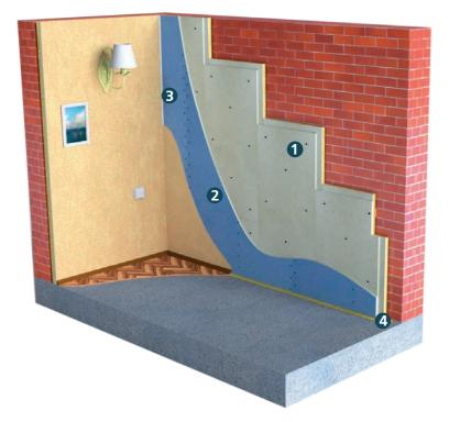
△R<sub>w≈</sub>18 additional airborne noise insulation
