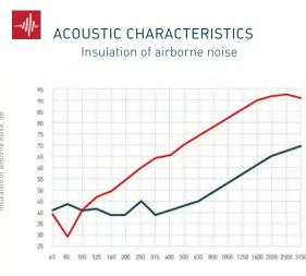
120 mm brick wall 120 mm brick wall + ZIPS-4 43 mm + gypsum plasterboard 12,5 mm
